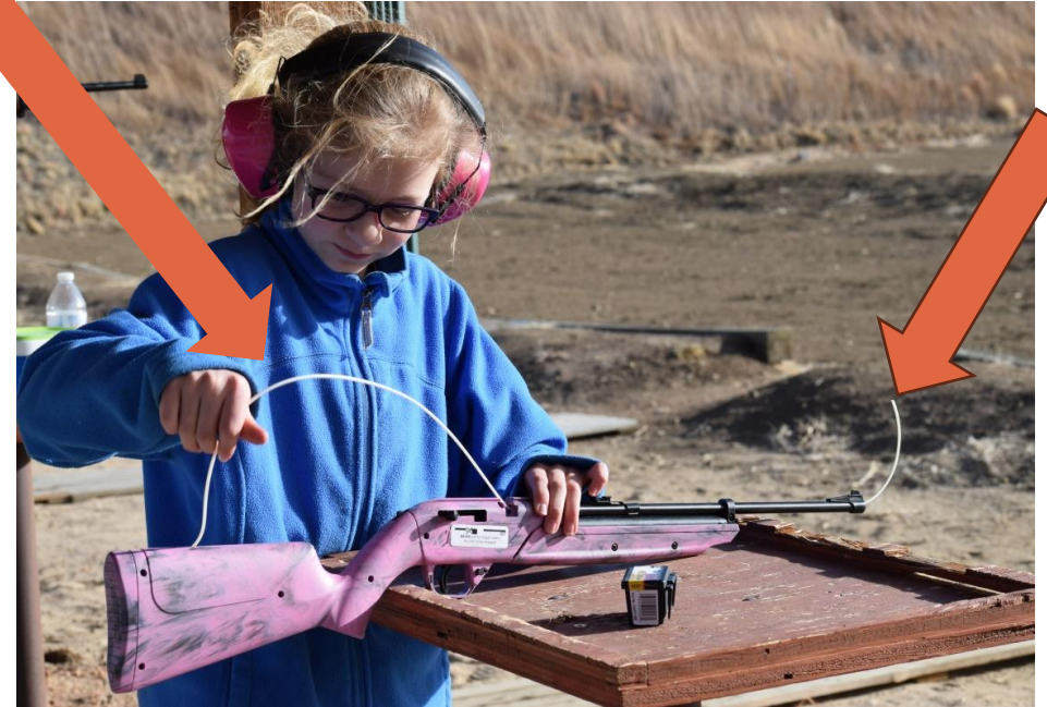
An example of a CBI being inserted into a firearm. You can see it in the action as well as coming out the end of the muzzle.
